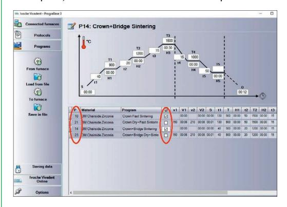
9. Save programs to furnace. In the Programs field, enter the program number to save to furnace, e.g. 10, 14 (Or if only one program is desired, just this single program number to save)
